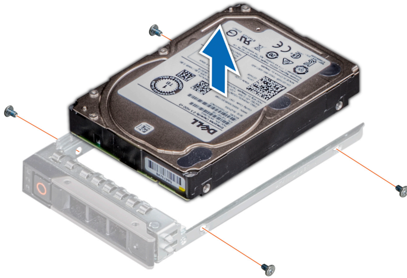
Figure 63. Removing the drive from the drive carrier
