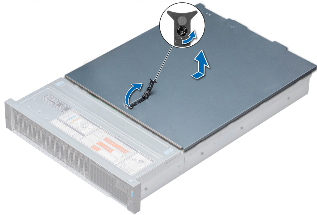
Figure 25. Removing the system cover
