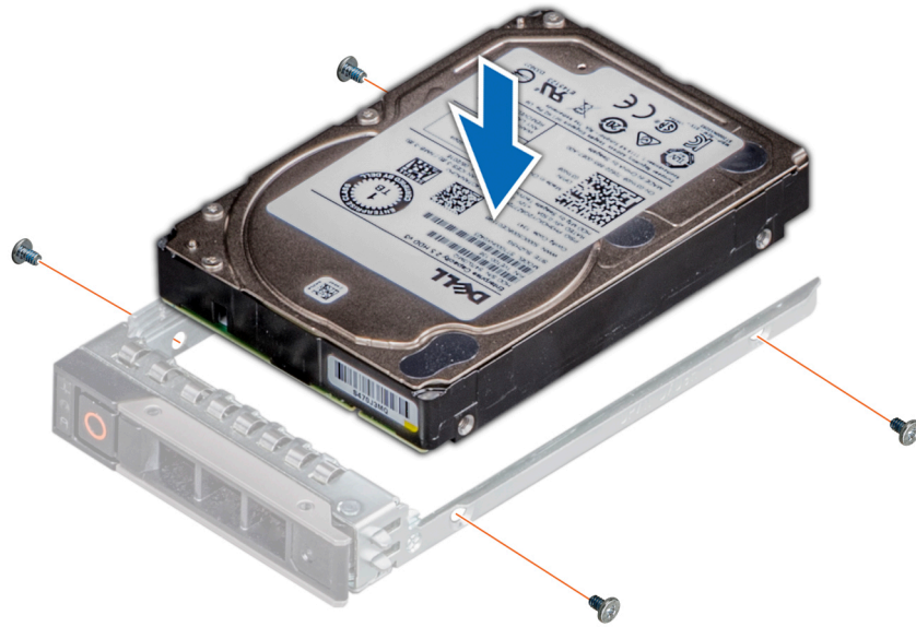
Figure 64. Installing a drive into the drive carrier
