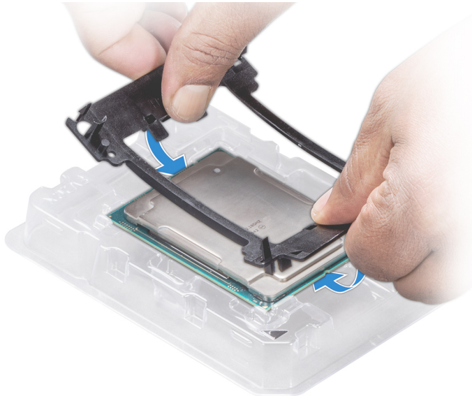
Figure 75. Installing the processor bracket
